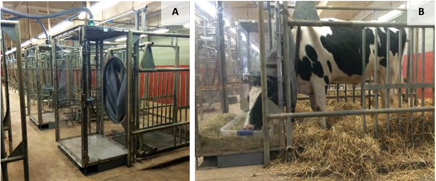
Figure 1. Panel A shows the unoccupied ventilated head boxes positioned side-by-side at the OSU Nutrition and Physiology Center. Panel B shows a Holstein heifer consuming feed during a gas emissions collection period.
