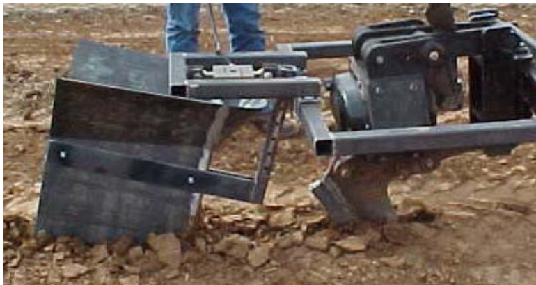
Figure 22. Shield Pulling Out of Ground during Testing
