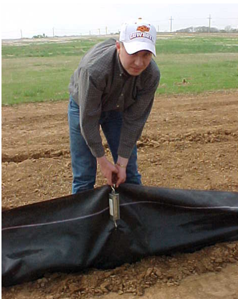
Figure 30. Spring Scale Testing to Determine the Force Required to remove Fabric from the Soil
