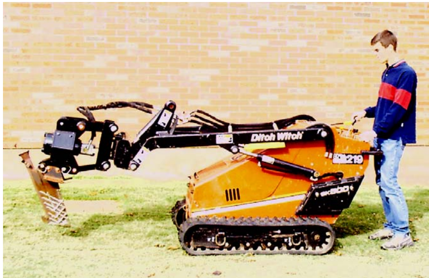
Figure 12. Ditch Witch SK500 with Vibratory Plow Attachment
