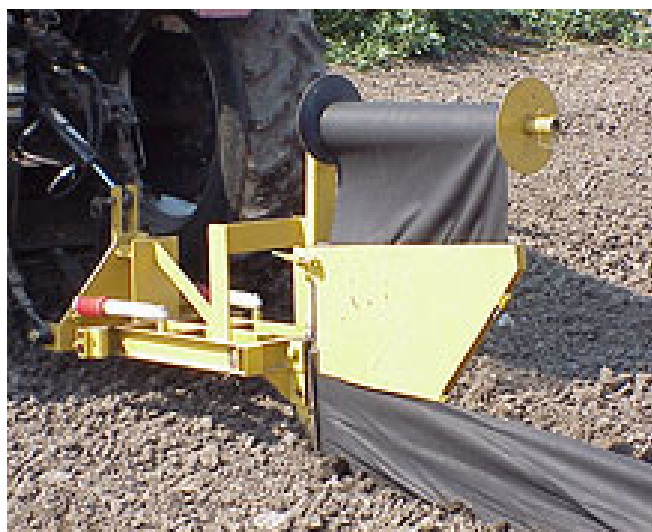
Figure 7. McCormick Silt Fence and Waterway Fabric Installation Plow (McCormick, 2003)
