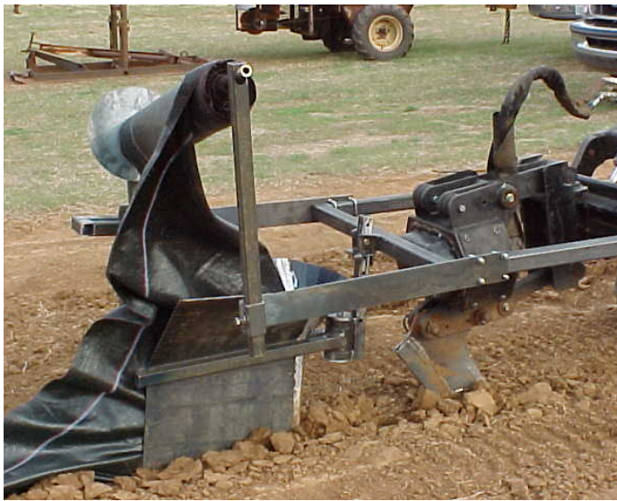
Figure 27. Adjustable Frame to Find Proper Fabric Roll Location and Orientation
