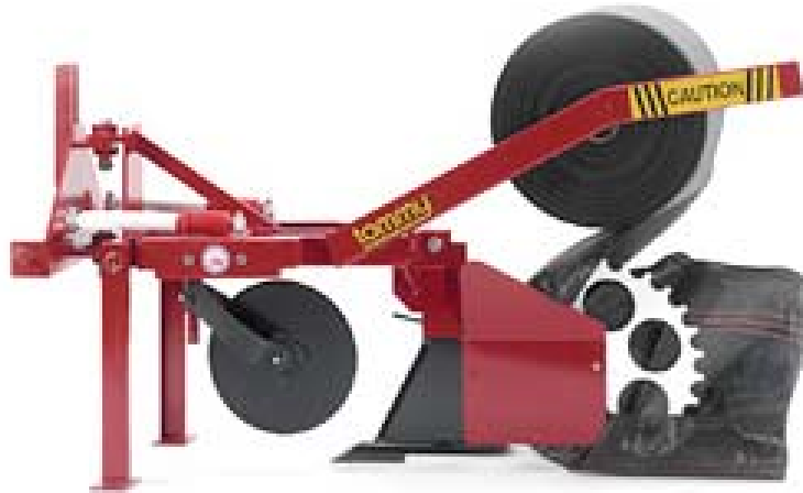
Figure 6. Tommy Silt Fence Machine (Tommy, 2003)
