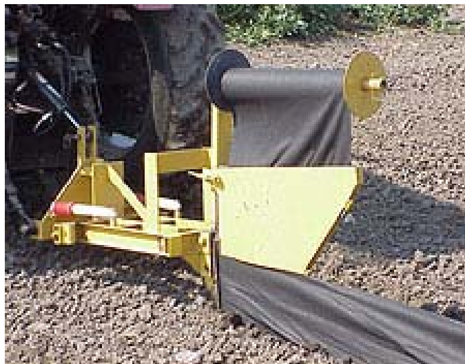
Figure 7. McCormick Silt Fence and Waterway Fabric Installation Plow 6
