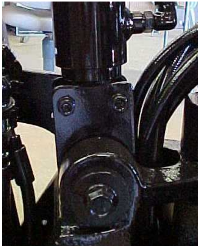
Figure 19: Cylinder stop preventing full retraction.
