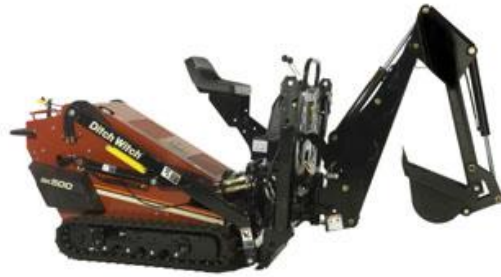
Figure 5: Ditch Witch SK500 with BradCo backhoe attachment.
