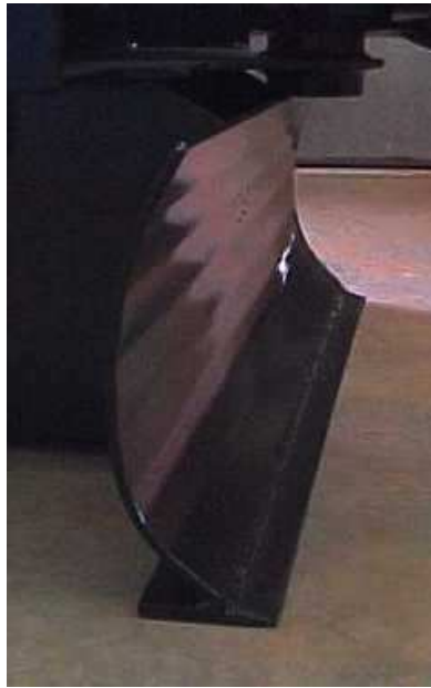
Figure 16: Backfill blade with cutting edge.
