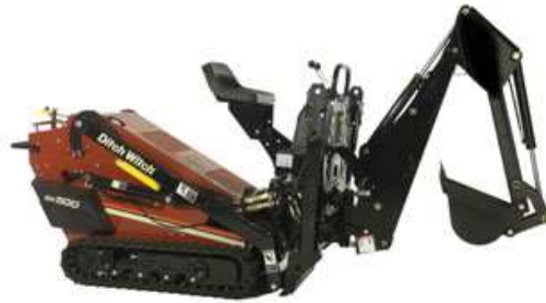
Figure 5: Ditch Witch SK500 with BradCo backhoe attachment.
