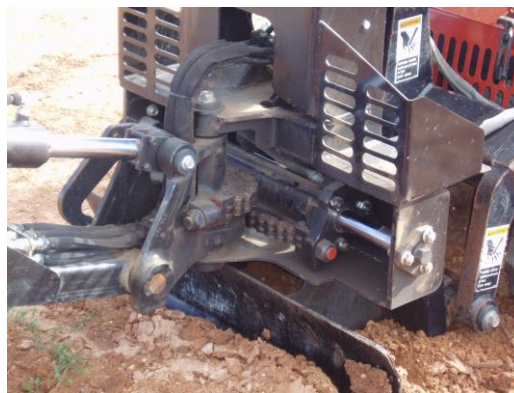
Figure 2: Backfill blade built in to main frame of backhoe.
