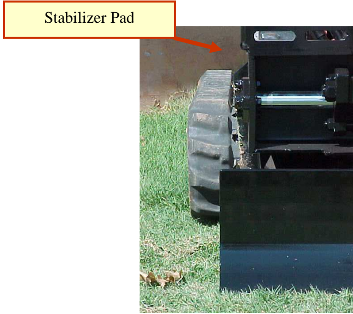
Figure 14: Stabilizer in folded up position inside the edge of the blade.
