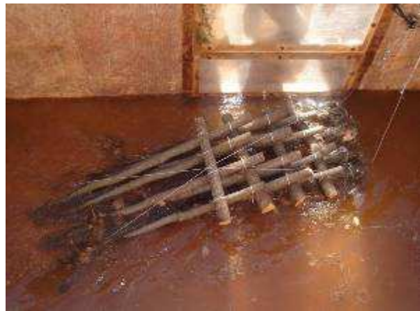
Figure 5 LWDS Model in Flume
