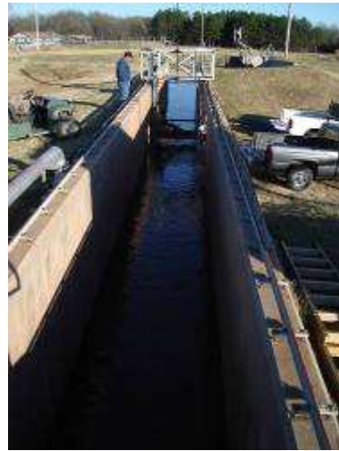
Figure 2 Large Concrete Flume at USDA-ARS Hydraulics lab
