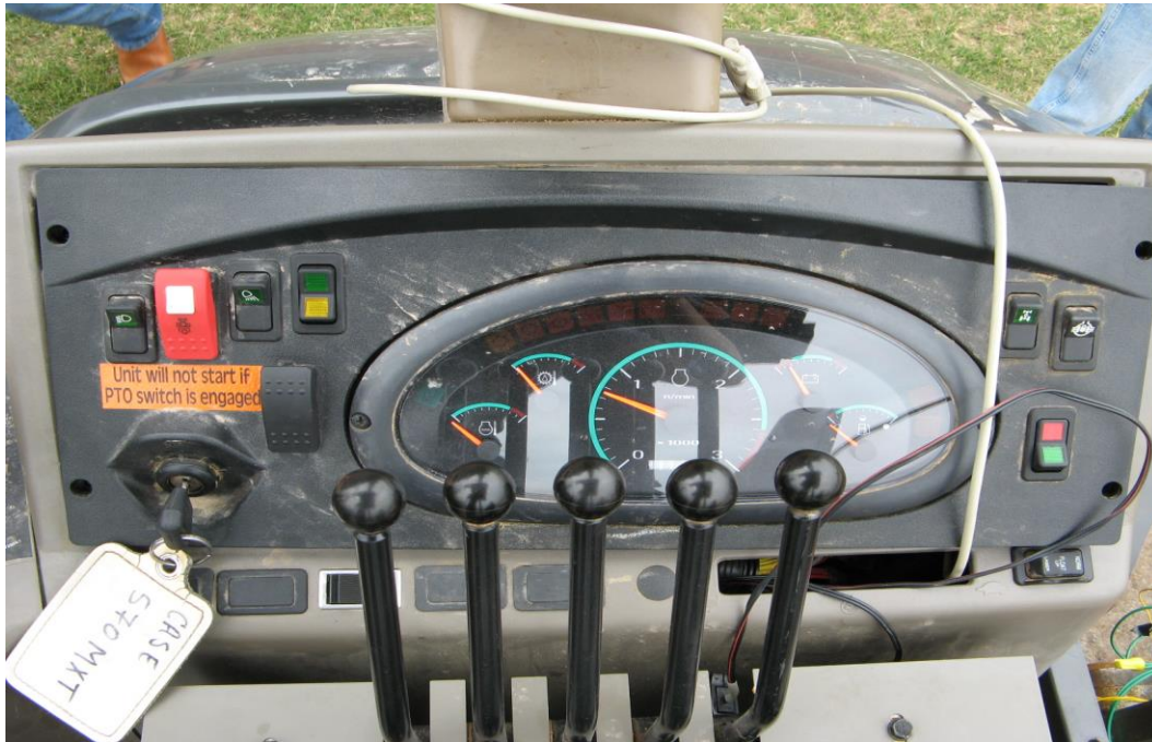
Figure 11. Control panel with 3 new switches added by Nexus Controls.
