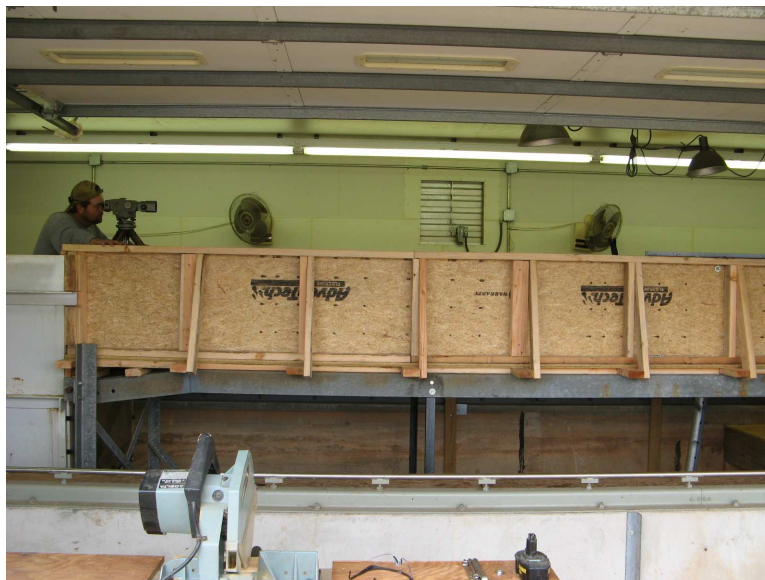
Figure 18. Surveying equipment being used to ensure levelness of point gage within 1/1000 of a foot.
