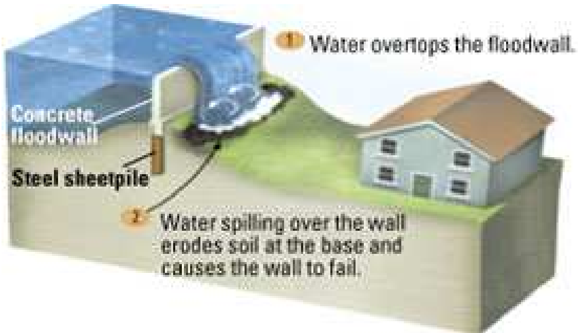
Figure 2. An example of the dangers of floodwall overtopping and scour. (Source: http://hsgac.senate.gov/_files/Katrina/Preliminary_Report.pdf )
