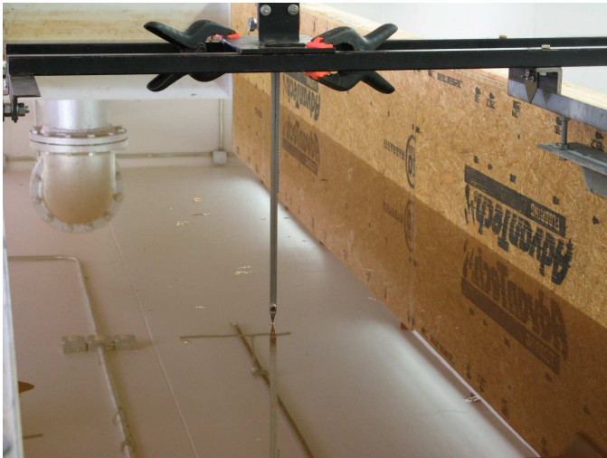
Figure 21. Point gauge at zero location, when flow was stabilized.
