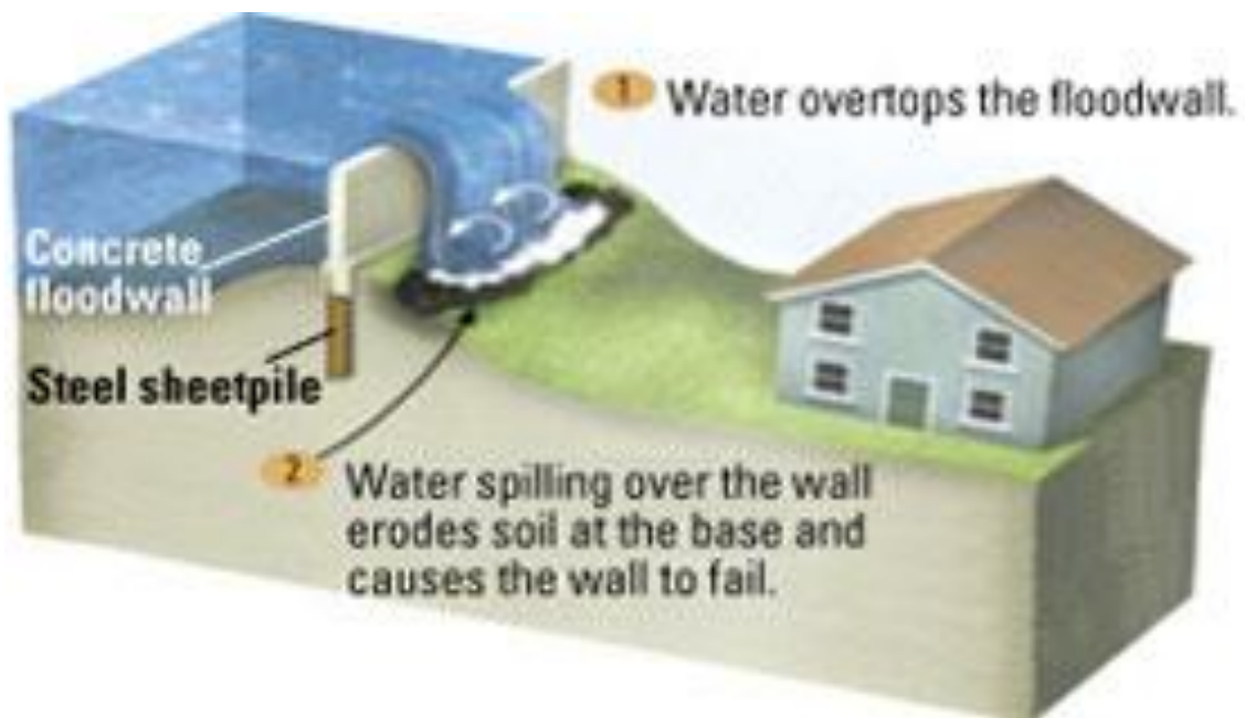
Figure 2. An example of the dangers of floodwall overtopping and scour.
