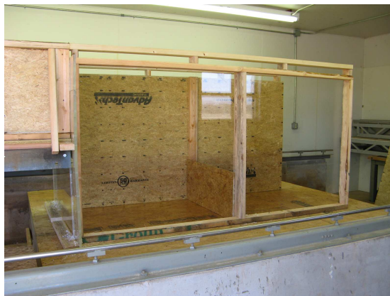
Figure 15. Completed rock box used for housing experimental materials.
