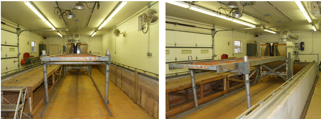
Figure 12. Pre-existing flume support structure and drainage basin.
