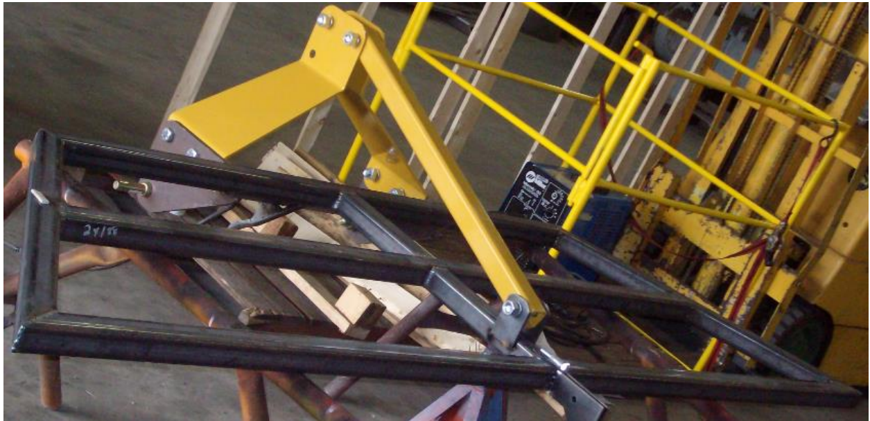
Figure 20: New Frame with Original 3 Point
