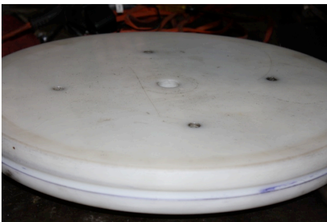
Figure 5: plunger used to force dough out of the bottom of the device
