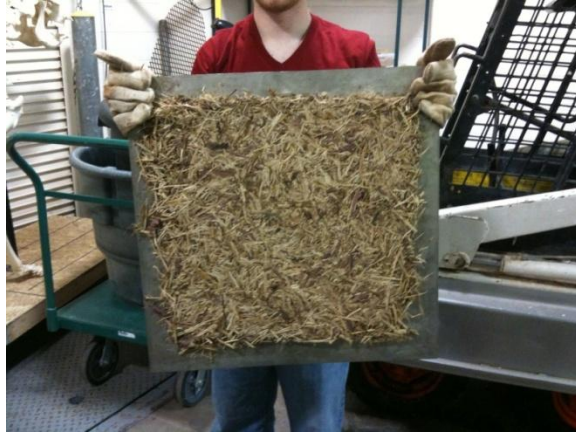
Figure 23. Mulch tile stuck to sheet after being pressed at 250°F.
