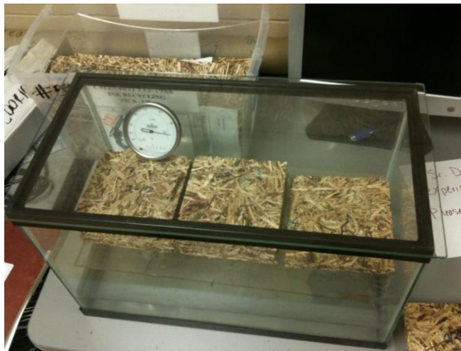
Figure 17. Relative humidity test setup, with hygrometer and mulch inside of the fish tank.
