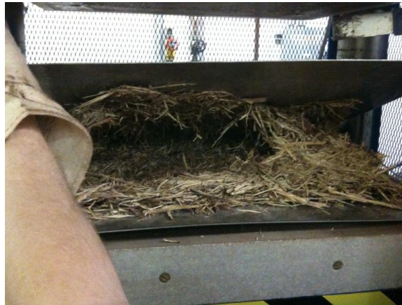
Figure 22. Mulch stuck to stainless steel sheets in heat press.
