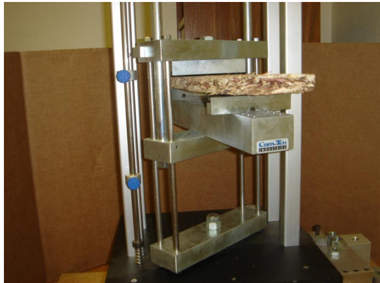
Figures 19 and 20. Universal Testing Machine used to test MOR of mulch tiles.
