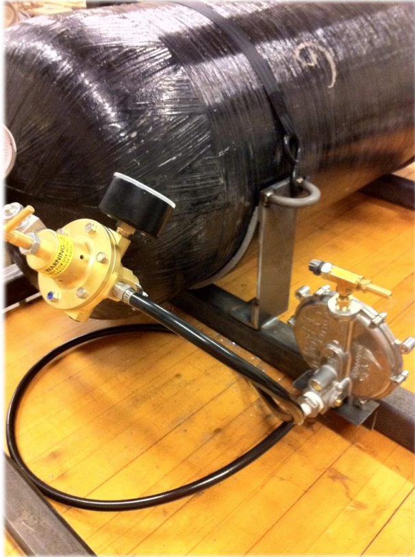
This photo shows the connection between the high-pressure regulator and the low-pressure regulator.
