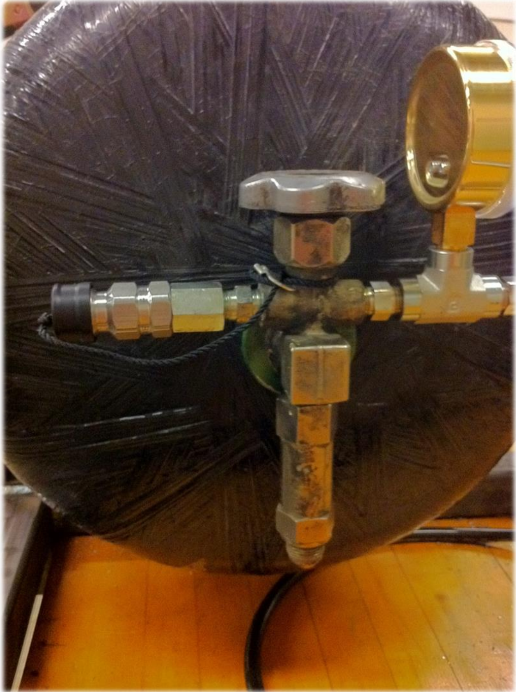
This shows the refuel nozzle, the tank shut off valve and the thermal relief valve.
