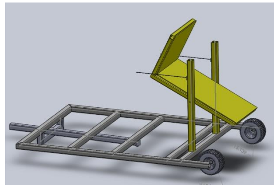
Figure 5: Releasing System – Releasing Position
