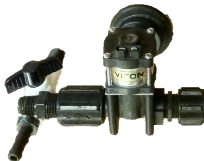
Figure 44. Viton solenoid valve for cleanout cycle.
