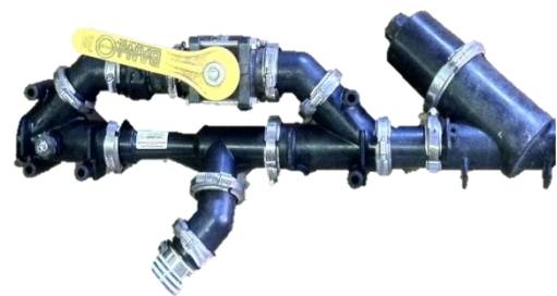
Figure 42. Venturi test stand with bypass.
