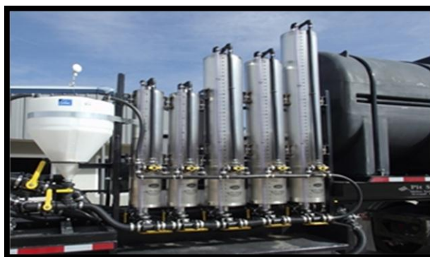
Figure 5. The JD Skiles pit-stop platform uses a volumetric measuring system.
