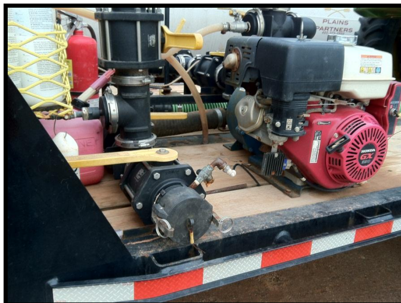
Figure 58. Manual primers help bleed air in hoses.
