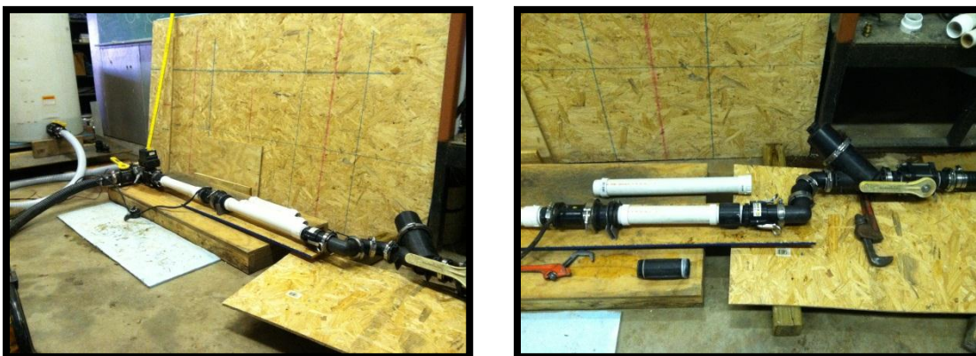
Figure 32. Measuring flowmeter error with regarding to flow uniformity.
