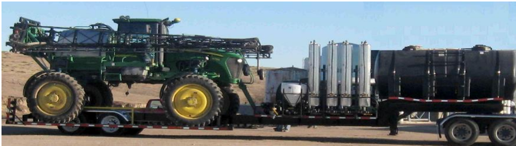
Figure 2. Tank, batch mix, and sprayer transport trailers.
