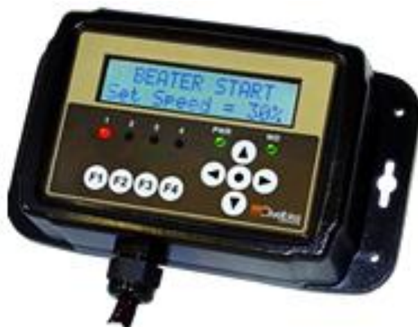
Figure 28. A potential development HMI with a robust housing and digital screen.
