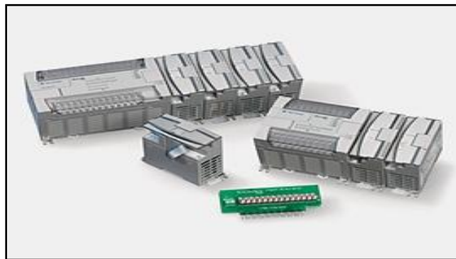
Figure 18. Allen-Bradley 1762-L24BWA programmable logic controller for algorithm development.
