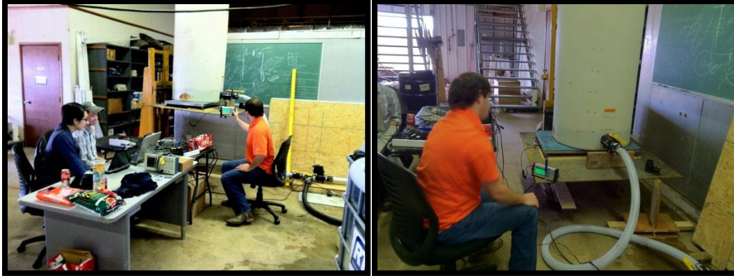
Figure 31. Performing metering accuracy tests as a function of height of head. Flow Conditioning and Piping Geometry
