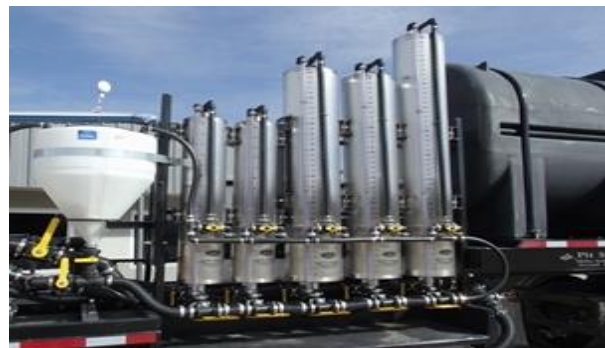
Figure 5. The JD Skiles pit-stop platform uses a volumetric measuring system
