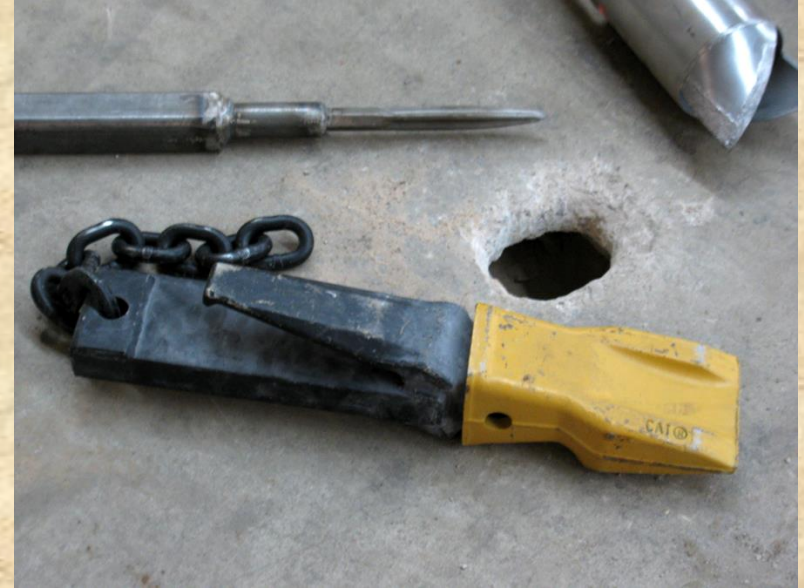
Bulldozer tooth and spike tooth are used to chip away rock layers
