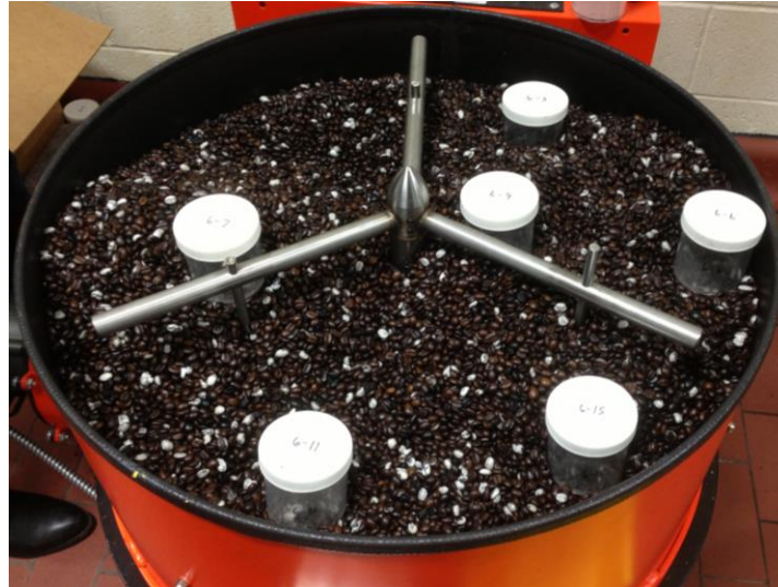
Figure 7: Arrangement of Sampling Cups, Prototype Arm.
