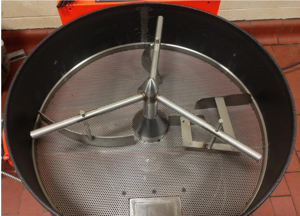
Figure 13: Prototype Rotary Arm in Model Cooling Bin
