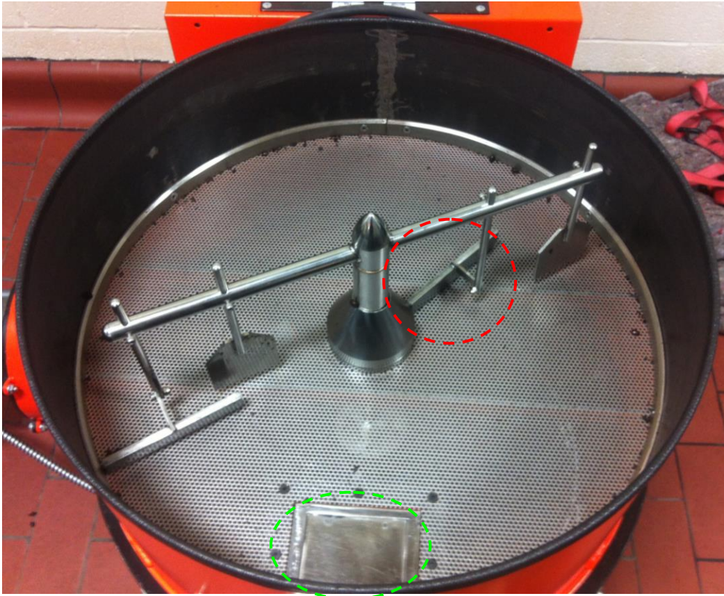
Figure 12: Default Rotary Arm in Model Cooling Bin. Exit hatch (circled in green) is in “closed” position.
