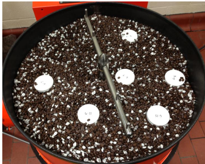
Figure 8: Arrangement of Sampling Cups, Default Arm.
