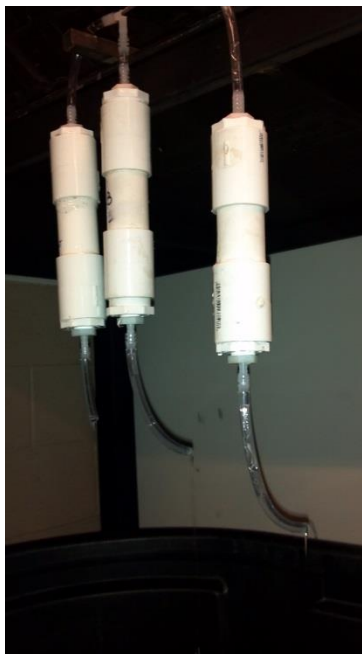
Figure 3 - Small modules filtering with gravity as driving force.
