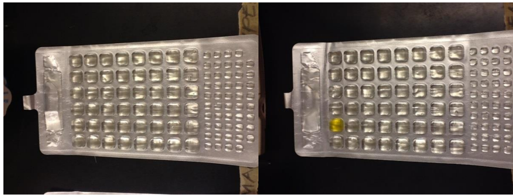
Figure 11 - Outflow samples three and four. One contaminated cell representing one bacterium per 100 mL sample.
