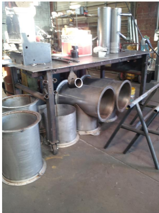
Figure 12. 300 Kilo Fire Tube Piping Completed.
