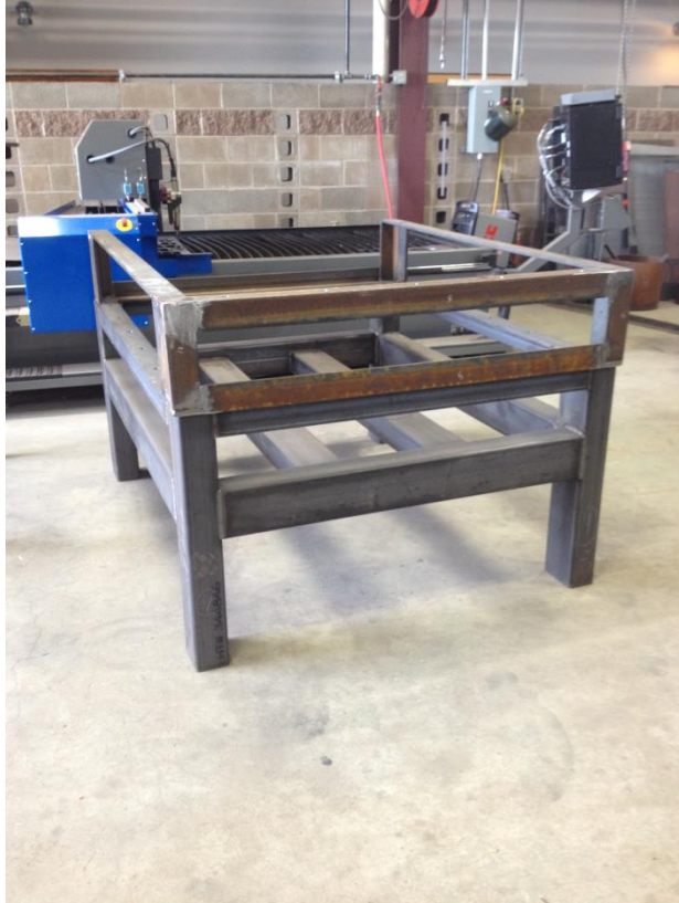
Figure 11. Completed 300 Kilo Upper and Lower Roaster Stand Assembly.
