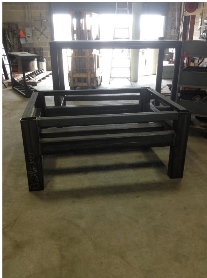
Figure 8. 300 Kilo Roaster Stand Fabrication Completion.
