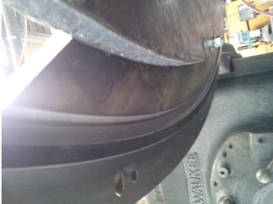
Figure 15. Up close view of the face plate showing grooves to hold the drum.
