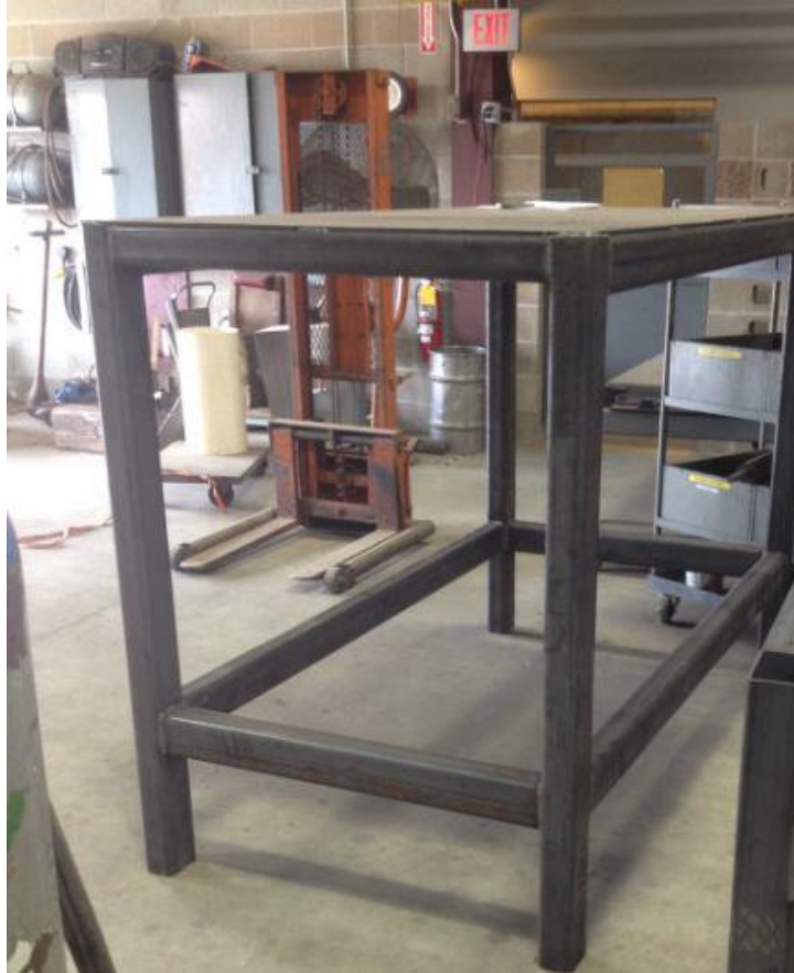
Figure 9. Completed Fire Tube Stand.
