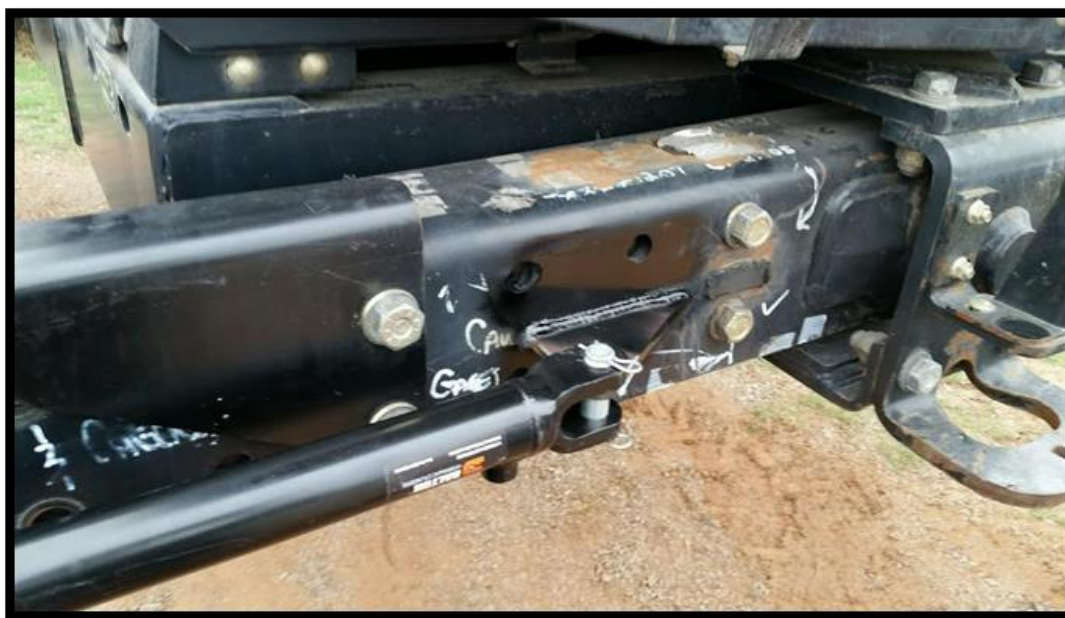
Figure 40. Bolt Covered by Cylinder on Rear Leg
