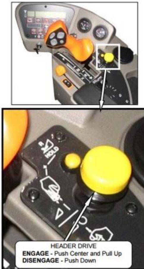
Figure 19-Header Engage/Disengage Switch from M155 operator's manual
