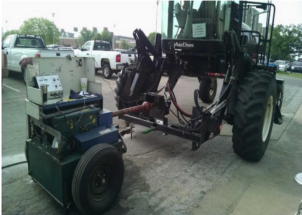
Figure 50: PTO Dynamometer Testing Setup
