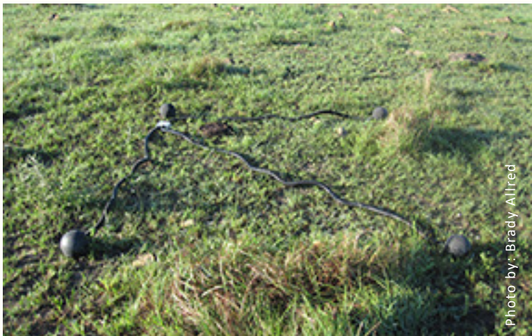
Black spheres used to collect operative temperature data.
