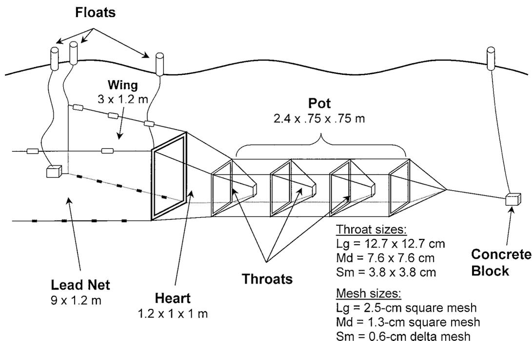
FIGURE 1.—Trap-net design used to test the effect of different mesh and throat size combinations on catch bias.
