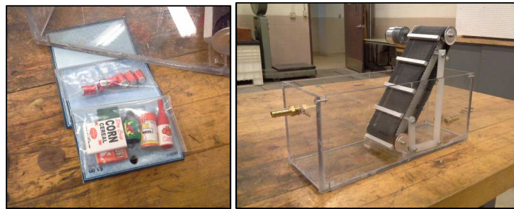
Figure 188: The “debris” used (Left) and the completed mechanical bar screens (Right)
