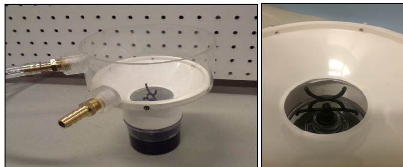
Figure 199: The grit removal chamber (Left) and the mixer impeller (Right)
