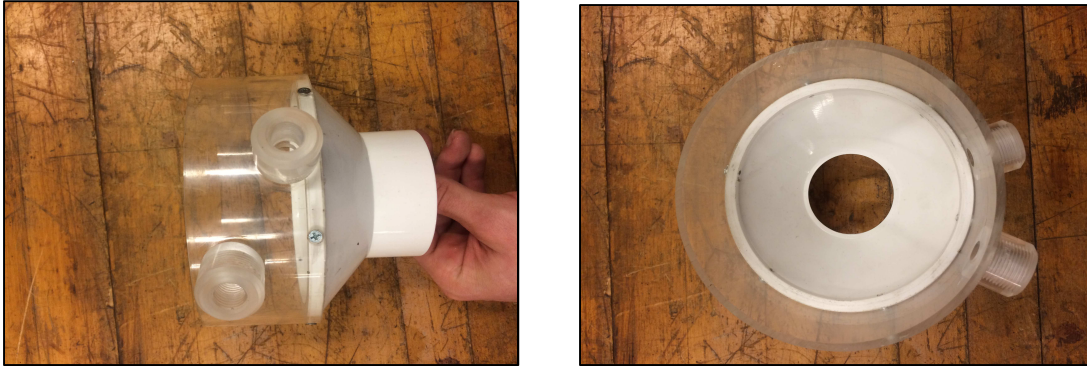
Figure 5: Profile (Left) and plan (Right) view of grit removal basin model. As shown, the water flows in through the higher inlet and, after traveling around the circumference of the basin, exits through the lower outlet.
