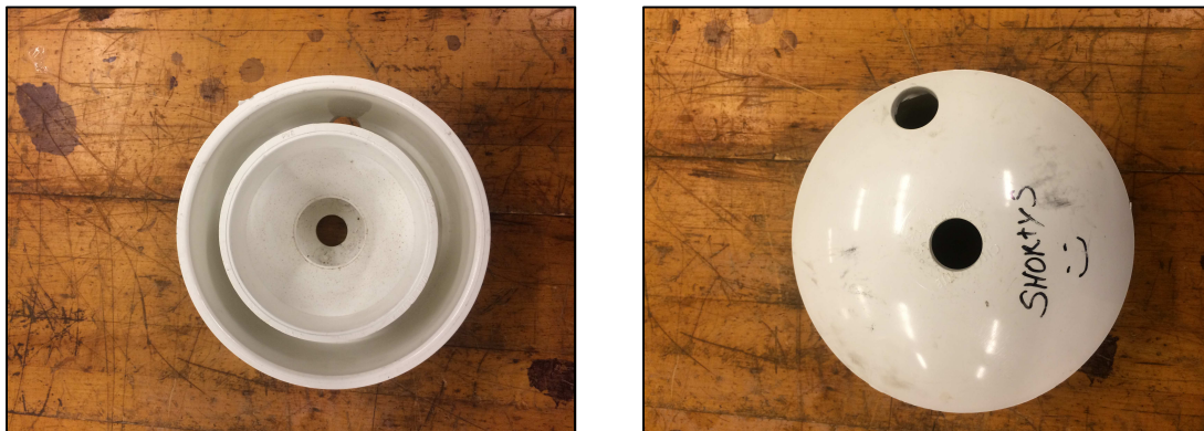
Figure 4: Top (Left) and bottom (Right) view of clarifier model. The inner chamber is a PVC reducer that was attached and sealed to the wall of the PVC end cap. Inlet (center) and outlet (rim) holes can be seen.
